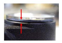
Now attach the new glass with adhesive. (for example: Loctite 401 or silicone adhesive Dreibond)
