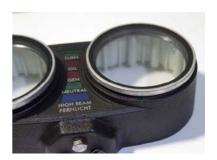
Clean up the outer edges of the raised lip with a file or sandpaper until you are able to push the new glass onto the protrusion.
