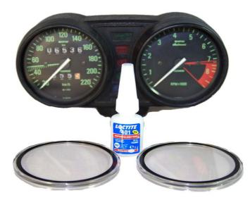
Disassemble the instrument cluster to the point where you have an empty housing. Remove the rubber visors from the front to expose the aluminum rings.
